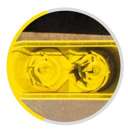
Counter-knives in the mixing tank: they ensure clean cut of fibrous products
